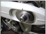
2) On models where the swing arm is recessed, install the spacer provided. If your swing arm is flat leave the spacer out.
