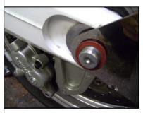
3) Install the new plate bracket and fiber washer. The washer will keep the plate from getting scratched up. Tilt the plate to the angle you want.
