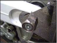
3) Install the axle nut and torque to spec. Consult a service manual for proper torque spec.
