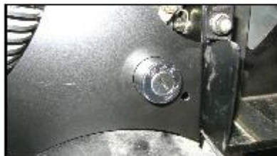
Fig. 4– Install ignition switch
