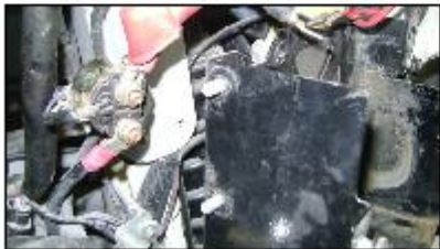
Fig. 2- Remove the 2 attaching nuts
