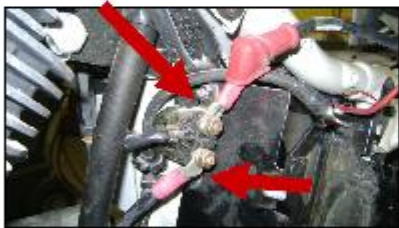
Fig. 2- Remove the 2 attaching nuts
