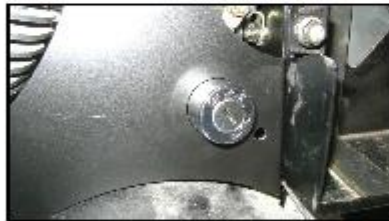
Fig. 4– Install ignition switch
