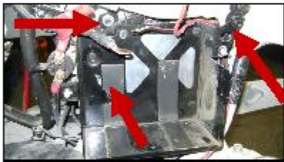
Fig. 1- Remove the 3 bolts
