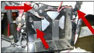
Fig. 1- Remove the 3 bolts
