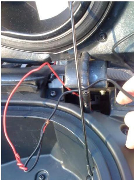
Twist the black LED wire a few times to make sure it doesn't come undone on the way through the hole. Make sure both wires are on the back side of that cable holding the trunk lid.
