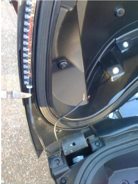
Left side done. Now cut off the short wire (you did end up with the short wire on this side, right?) and put a dab of silicone on the tip of that wire to seal it.
