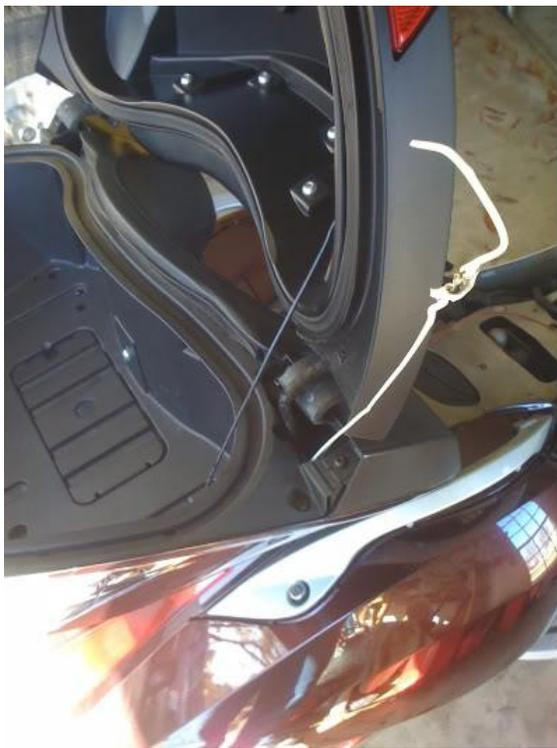
(Fig. 4) It will come out here. (Note) Make sure that big gray wire is *behind* the big flat tab or the seat will not go back on right later.
