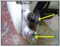
Remove stock controls on left and right hand side. Remove shift rod bolt from the shift lever. On 4&5 inch extension kits remove the stock banjo fitting from the rear master cylinder located on the right side peg. CAREFULLY remove the stock rubber reservoir hose. BE CAREFUL NOT TO BREAK THE PLASTIC LINE FITTING. Install the new extended hose with the new squeeze clamps.
