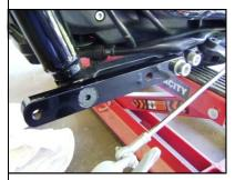
Install the right & left side extensions using one 10mm x 50 flat head socket bolt and one 10mm x 25 socket bolt. \*The front left hand side bolt may be hard to get in. It may be necessary to gently pry the frame back into place for the bolt to line up.
